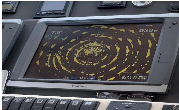
FIGURE 1.3 Photograph of the display of a shipboard radar operated in a U.K. wind farm.
