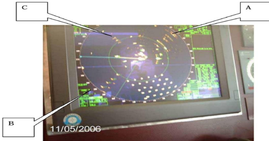
Marico FIGURE 2.10 Illustrative plan position indicator display for magnetron-based radar from the Kentish Flats experiments, where the points A, B, and C highlight the phenomena of multiple target echoes due to wind turbine generator–radar interaction, and Radar screen near 5 turbine Block Island RI 5 turbine project.
