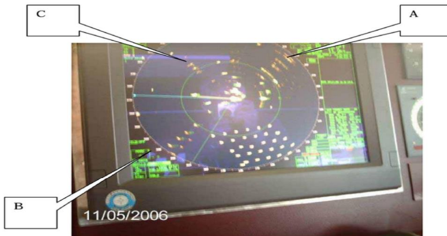
Marico FIGURE 2.10 Illustrative plan position indicator display for magnetron-based radar from the Kentish Flats experiments, where the points A, B, and C highlight the phenomena of multiple target echoes due to wind turbine generator–radar interaction
