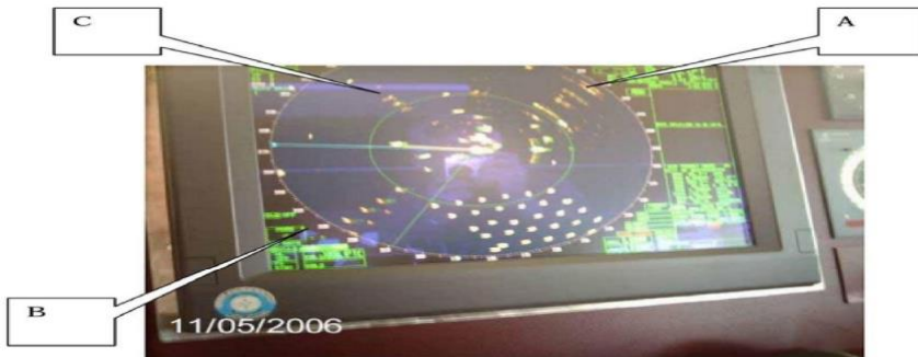
Marico FIGURE 2.10 Illustrative plan position indicator display for magnetron-based radar from the Kentish Flats experiments, where the points A, B, and C highlight the phenomena of multiple target echoes due to wind turbine generator–radar interaction, and Radar screen near 5 turbine Block Island RI 5 turbine project.
